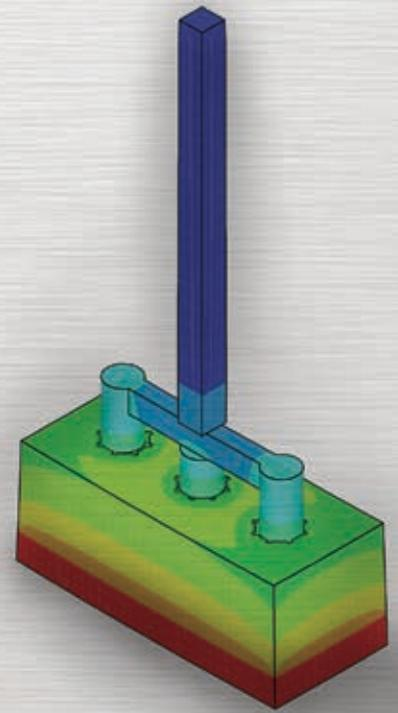
Thermo-electro-mechanical finite element analysis of an anode.
